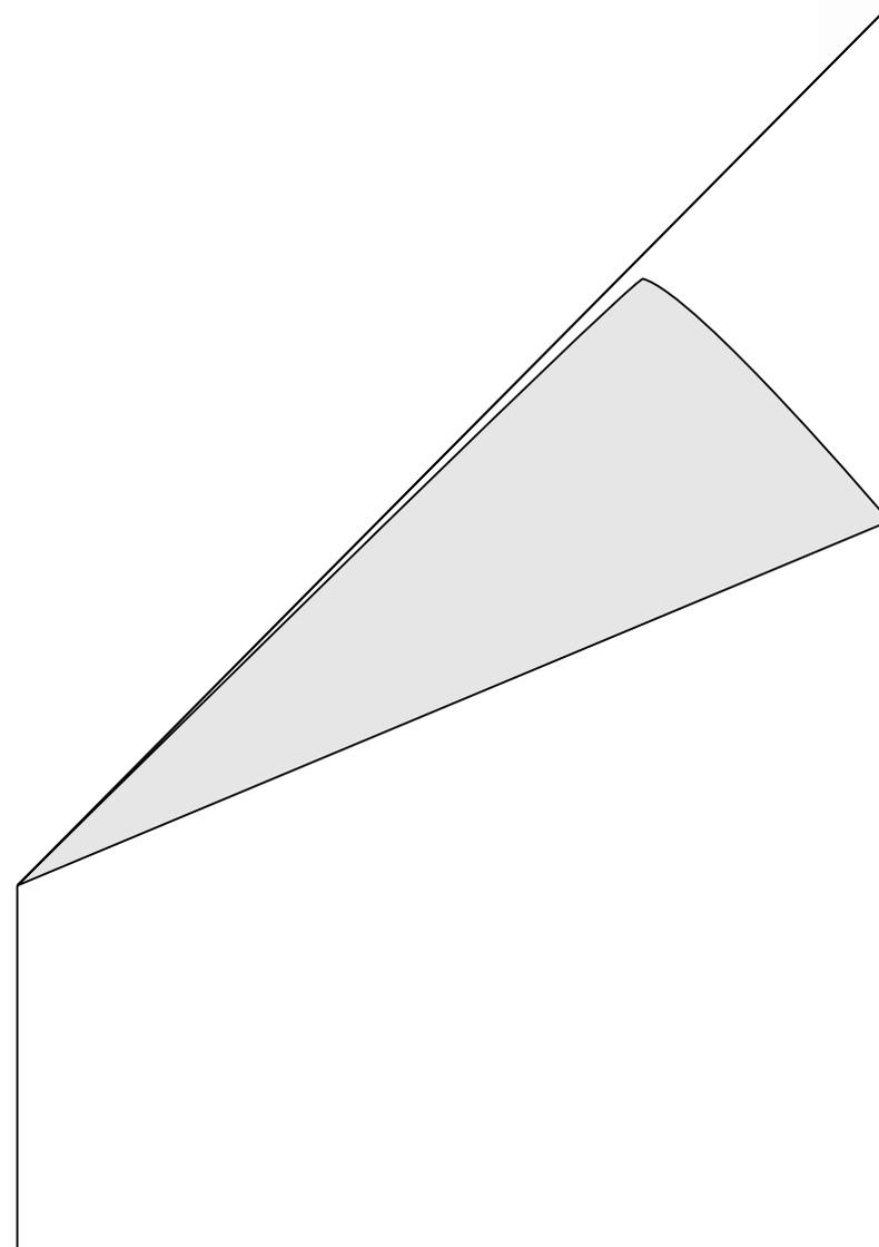
**Design Note:** This is one of the steps that makes the Paperang unique. The centerline cut makes it possible for the spars to overlap in the middle of the wing for strength. The curved cut in the trailing edge removes paper that cannot be accurately supported by the spars, increasing the aspect ratio at the same time. Use the full sized templates on the following page to help you cut the trailing edge.
