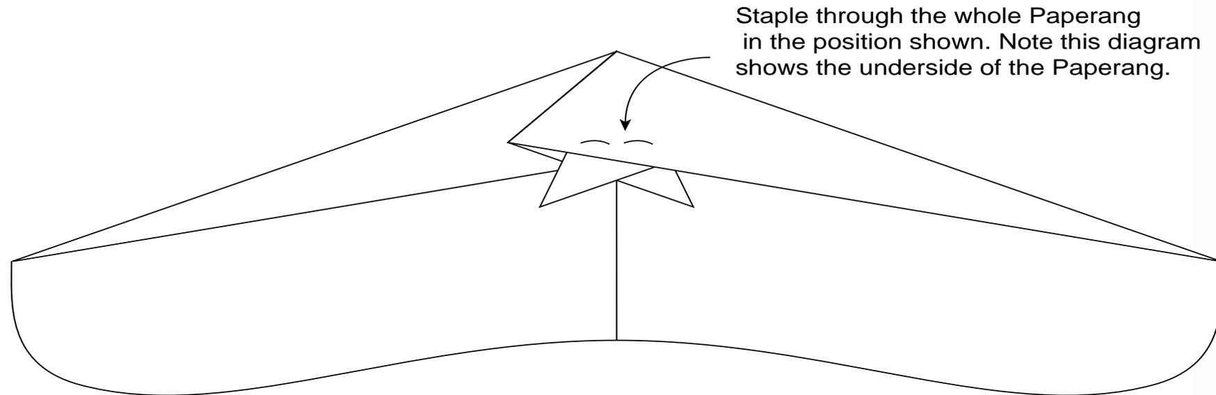
***Design Note:*** The performance of a Paperang is determined by its shape when you staple it. Please make sure that all the folds are equally flattened, and that both wings are straight and symmetrical. Place the Paperang in the jaw of the stapler and grip lightly. Check everything is in align-
